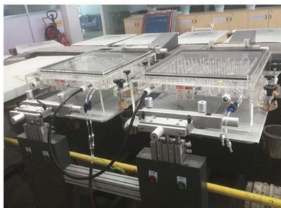
◆ 植绒机 (植毛面积350x450mm) Flocking machine (Flocking area350x450mm)
